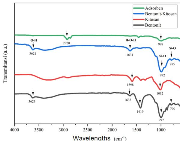
**Figure 2.** FTIR Spectra of Bentonite, Chitosan, Bentonite-Chitosan Composite and Bentonite-Chitosan Adsorbent After Contact with Used Lubricating Oil
