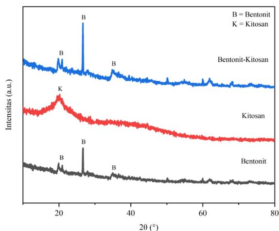
**Figure 1.** Diffractogram of Bentonite, Chitosan, and Bentonite-Chitosan Composite
