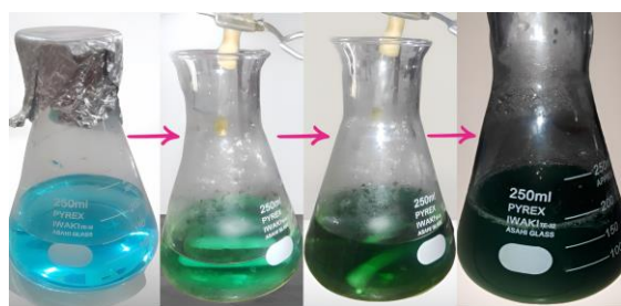
Figure 2. Color changes during the reaction between S. lappa root extract and Copper sulfate pentahydrate solution
