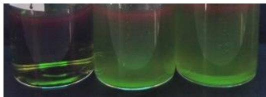
EML + anion under UV lamp (fluorescence on with green colour, no colour)
