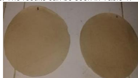
Figure 1. Sheets of green ampel bamboo pulp handsets
